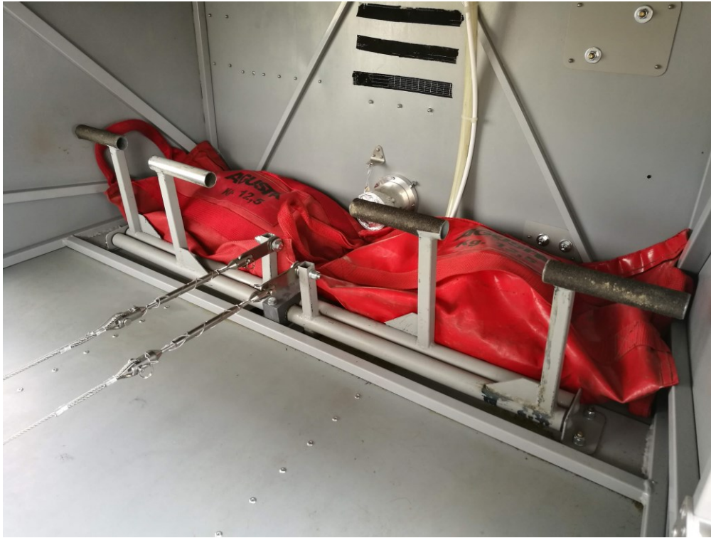
Figure 5.11: Two ballasts behind the pedals
