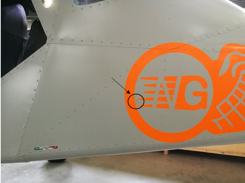
Figure 2.4: Particular of the static pressure probes
