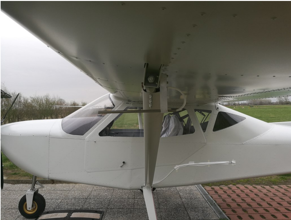
Figure 5.2: Final configuration – Particular of the total pressure tube
