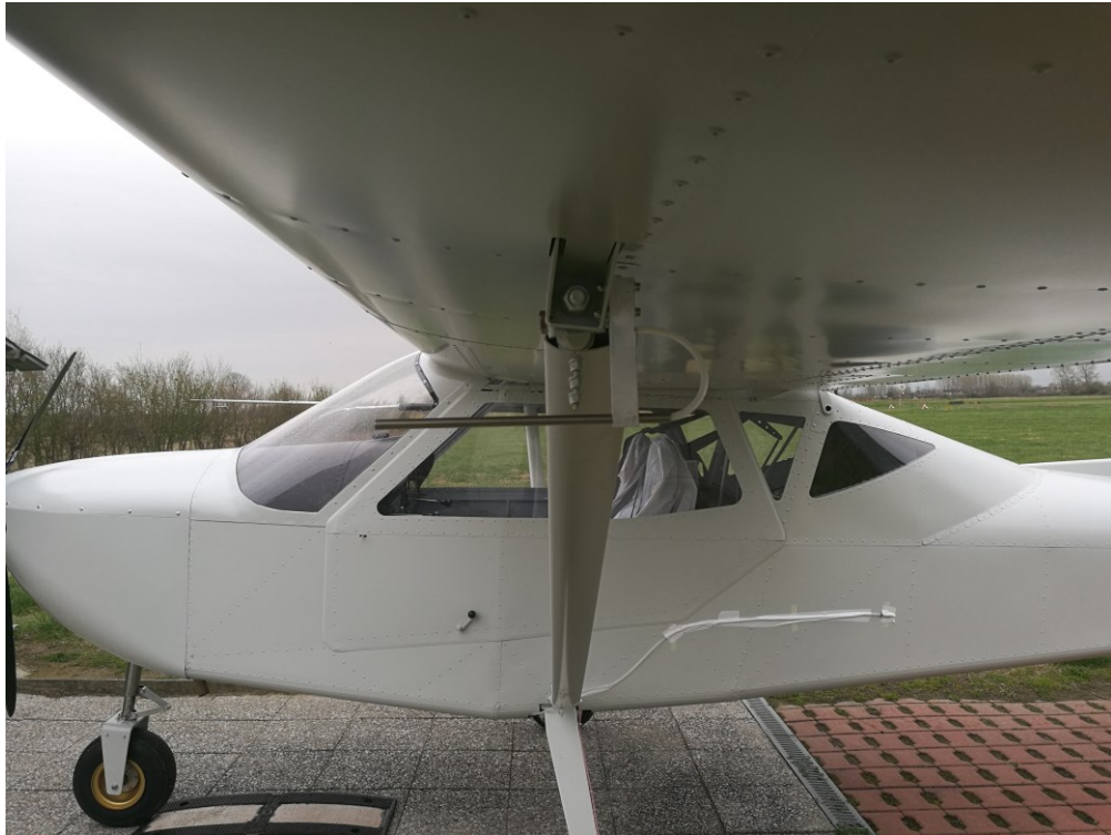
Figure A.0.24: G70 new Pitot tube correctly installed
