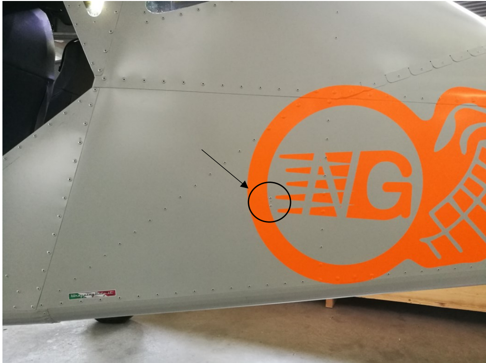
Figure 5.3: Final configuration – Particular of the static pressure probes
