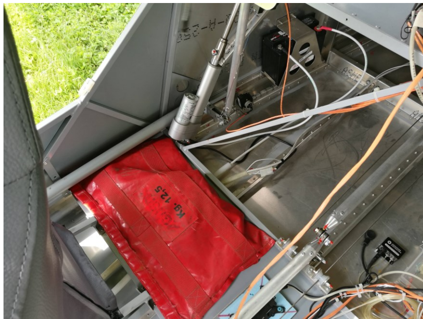
Figure 5.13: Ballast behind passenger seat
