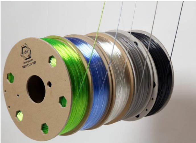
The Recycled and virgin Filaments are Provided by REFIL company. fully recycled ABS filament made from car dashboards and PET filament made from old PET bottles in Blue and Green colors, and fully Recycled PLA from white food packing. ( http://www.betterfuturefactory.com/project/refil/ )
