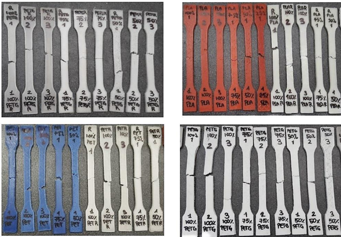
Fig.2. 14: This picture shows the results of tensile testing on different prints by different filaments.
