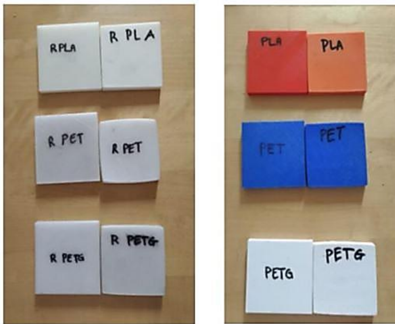
Fig.2. 13: This picture shows the comparison images of the specimens before and after the cycle in the climatic chamber
