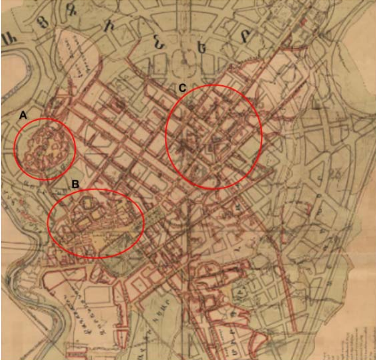
Figure 41: Tamanian's master plan superimposed on a previous map from 1920 to highlight the changes. Except the areas in three circles A, B, and C, he respected the existing urban texture created by Russians in 1856. He widened some streets to adapt it to a city of 150,000 inhabitants.
