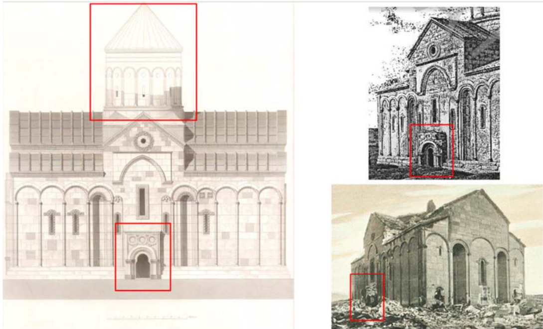
Figure 10: Left: The South elevation of Ani cathedral by Texier. Elevation differentiating the collapsed dome and the existing building. Meanwhile, the portal is depicted in original state. From Texier, 1842, Vol. I, plate XX. Top Right: A perspective view of the building drawn in the same expedition trip by Texier's team mate. The damaged portal is visible. From Texier, 1842, Vol. I, plate XVII. Bottom right: Photograph of the Ani Cathedral by Lynch. From Lynch, 1901, Vol. I, figure 72, opposite page 370.
