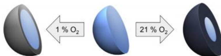
Figure 28. A schematic representation of a cobalt particle (light blue), as half sphere of average diameter illustrating the dependence of the formed oxide type (CoO: grey, Co 3 O 4 : dark blue) and the oxide layer thickness on the concentration of O 2 during the passivation.
