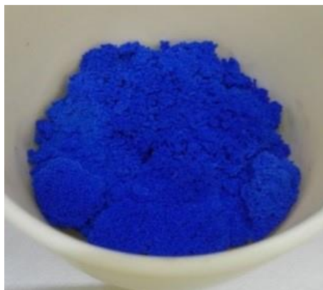
Figure 10. Image of the \gamma\text{-Al}_2\text{O}_3 support stabilized with \text{CoAl}_2\text{O}_4 species.
