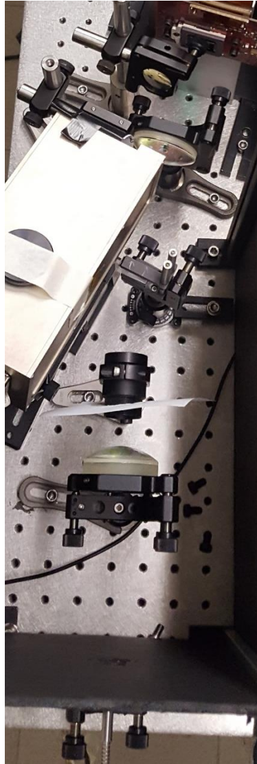
Fig. 18 Configuration_1 optical setup, in both figure the input beam from the fiber bundle is coming from the bottom of the picture, the first lens works as collimator D50 F100. Follows the aperture and the grating (squared optical elements). After the grating the beam is focused on the DMD ( The red element is the DMD electric board) . once the beam is reflected from the DMD in on state it enters the second branch, made up by the two lenses D25 placed on a different propagation plane, together with the Detector cage.
