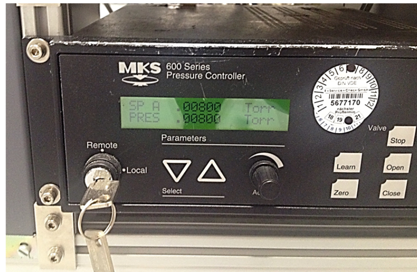
(b) MKS 600 Series pressure controller showing the fixed set point a and the pressure value measured in the chamber by baratron number 1
