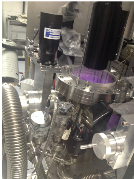
(d) GEC seen from its right side after switching the RF power on: plasma on
