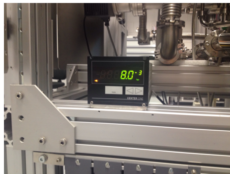
Figure 2.8: Read-out of the pressure measured by the combination of ionization manometer and Pirani gauge
