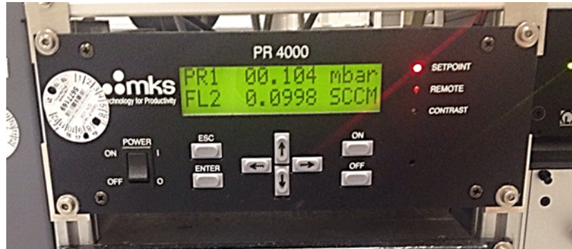
(a) MKS PR 4000 controller showing the pressure measured by the baratron connected to the for-vacuum line (number 3) and the gas inflow measured by the flow controller
