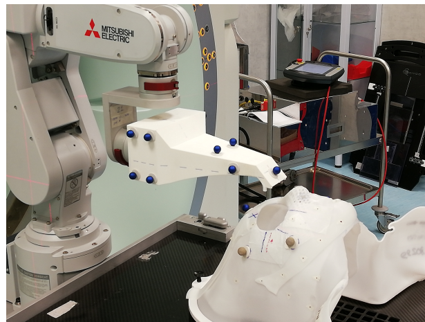
Fig. 4: ETS device connected to the positioning system (robotic arm) and thermoplastic mask in the TAC room.
