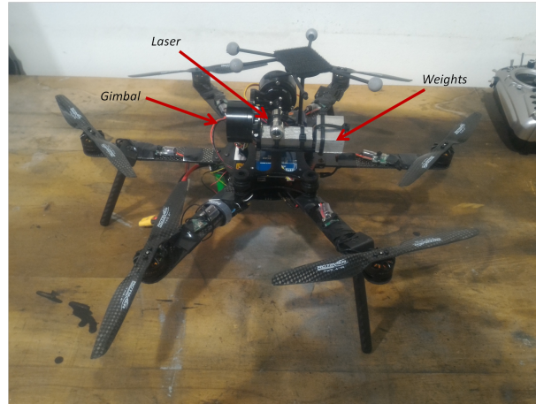
Figure 1.8: Laser targeting system mounted on Hexa2
