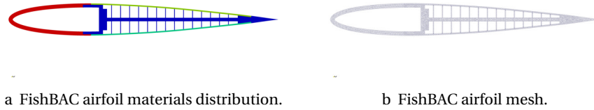
Figure 5.3 – FishBAC airfoil materials and mesh.
