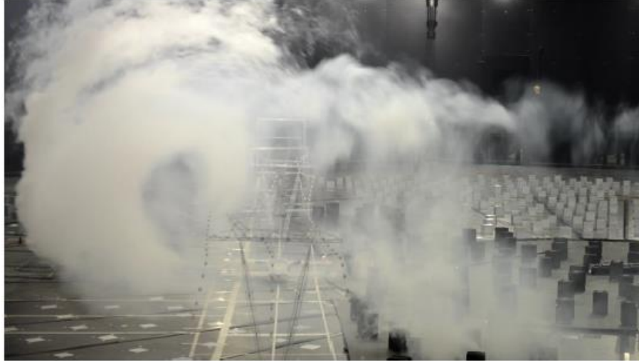
Figure 2-23: Typical downburst generated in WindEEE Chamber. Adapted from: (Elawady 2016)
