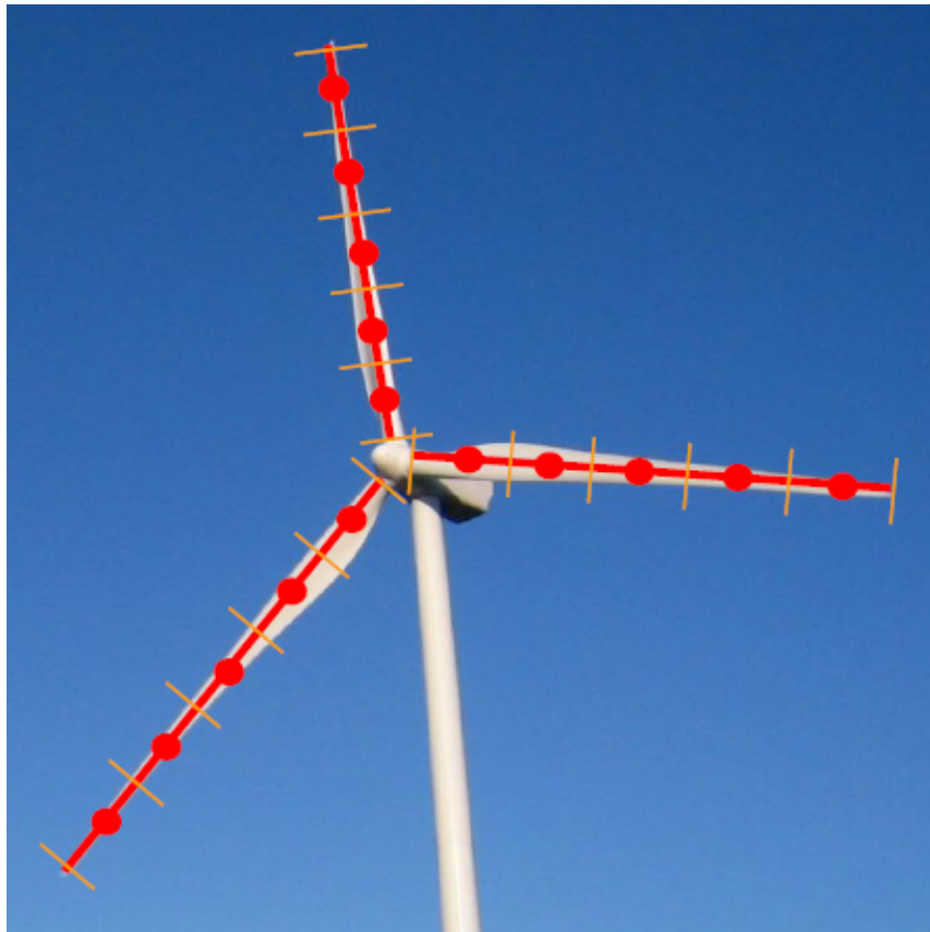
Figure 3.5: Actuator Line Model of a wind turbine rotor.
