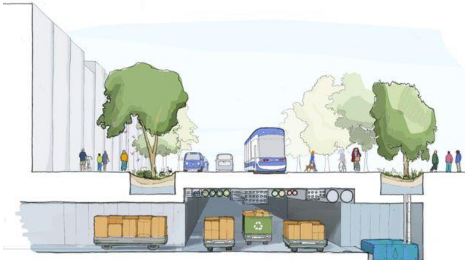
Figure 3.20: Utility channel concept art (Source: Sidewalk Toronto) [22]
