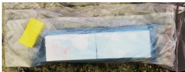
Figure 7.1 – Flexible polyethylene bag used for fracture tests in active environment.
