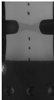
Figure 5.12 - Plastic zone ahead of the crack tips during a test on 0.5 mm thick DENT sample obtained from a bottle.
