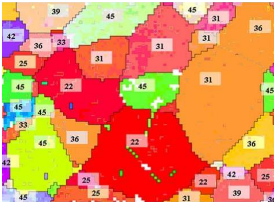
Figure 54: Estimated oxide layer thickness values (in nm) for each grain based on a color comparison to reference anodized samples which oxide layer thicknesses were obtained through spectrophotometry. Those values were superimposed on the crystallographic orientation map (from [79]). The scale is the same as the one presented on Figure 50.
