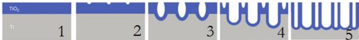
Figure 40: Different steps of the nanotubes growth (from [76]).
