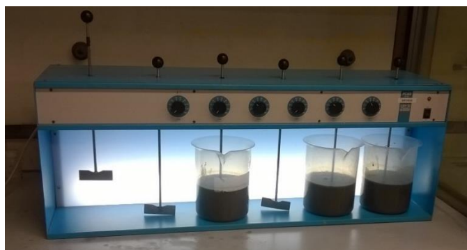
Figure 3.3 - Conditioning of the sludge by jar test in the laboratory.
