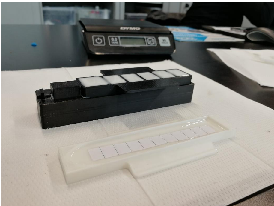
Figure 3-16 Silicone rubber injected inside the molds
