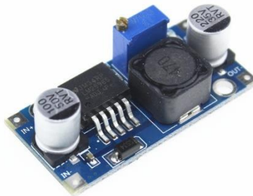
Figure 6-7 LM2596 switching voltage regulator
