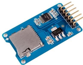
Figure 4-11 Mirco SD module for Arduino
