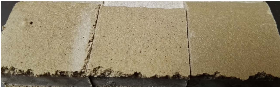
Figure 28. Membranes obtained from samples S_e (left) and S_c (middle) compared with a reference (right) from AkzoNobel.
