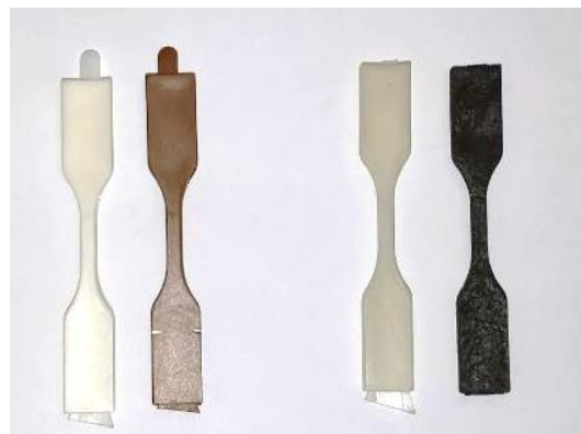
Figure 63 Effect of oxidation after exposure to the temperature of 190°C for 1416 hours, both in case of Later 4 G/30 (left) and Latamid 66 H2 G/30 (right)
