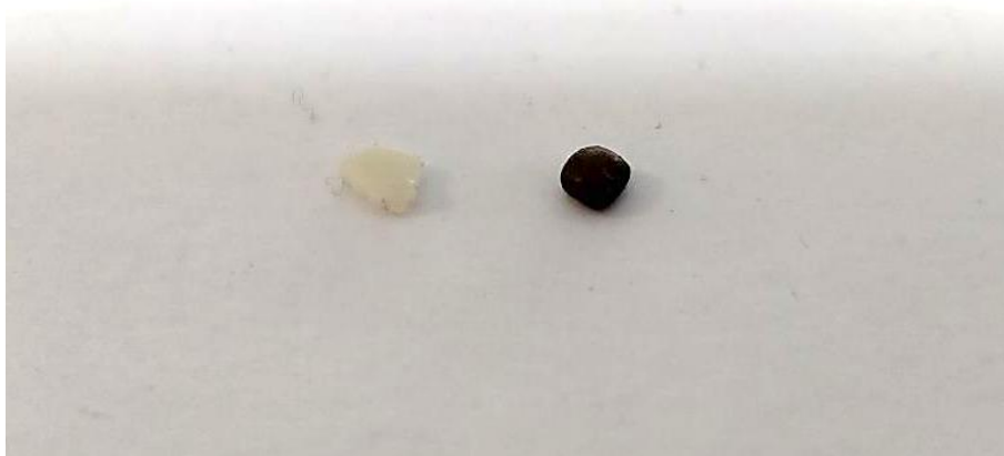
Figure 70 Comparison between an unaged Latamid 66 H2 G/30 sample and one subject to a heat ramp up to 300°C in a thermogravimetric furnace
