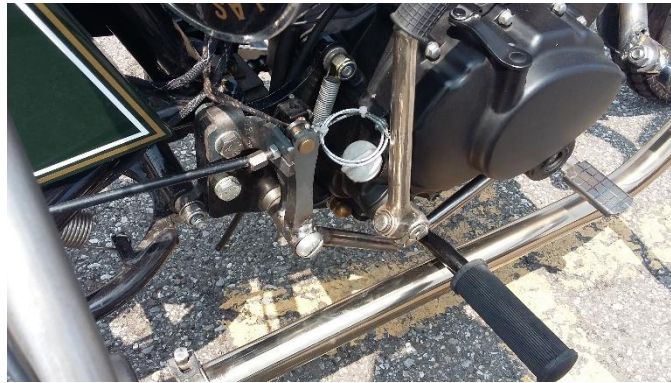
Figure 4-17 Coupling between rear and side brake system
