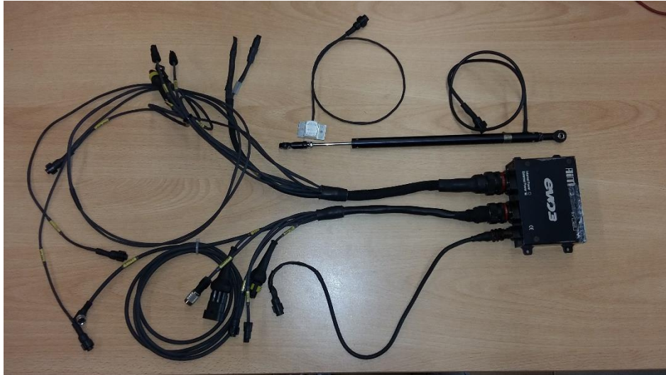
Figure 4-24 Acquisition Data system
