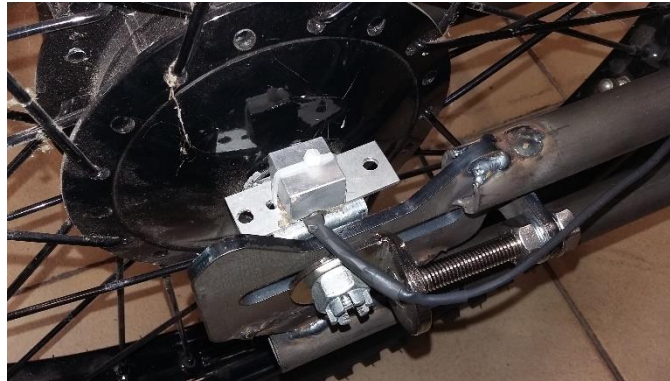
Figure 4-27 Side biaxial accelerometer positioning
