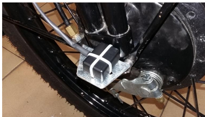
Figure 4-26 Front biaxial accelerometer positioning
