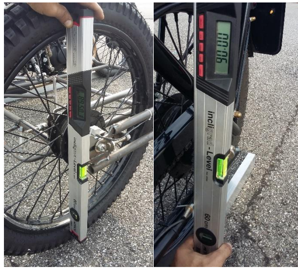
Figure 4-37 Camber angle check on the test track
