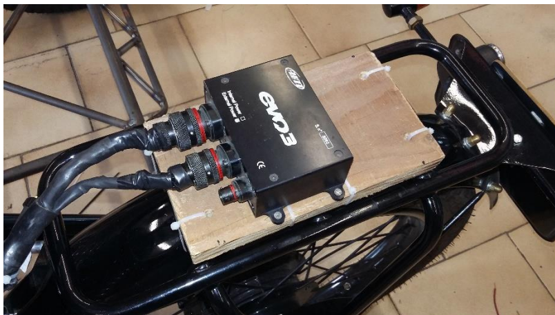
Figure 4-25 Data Logger positioning on the vehicle
