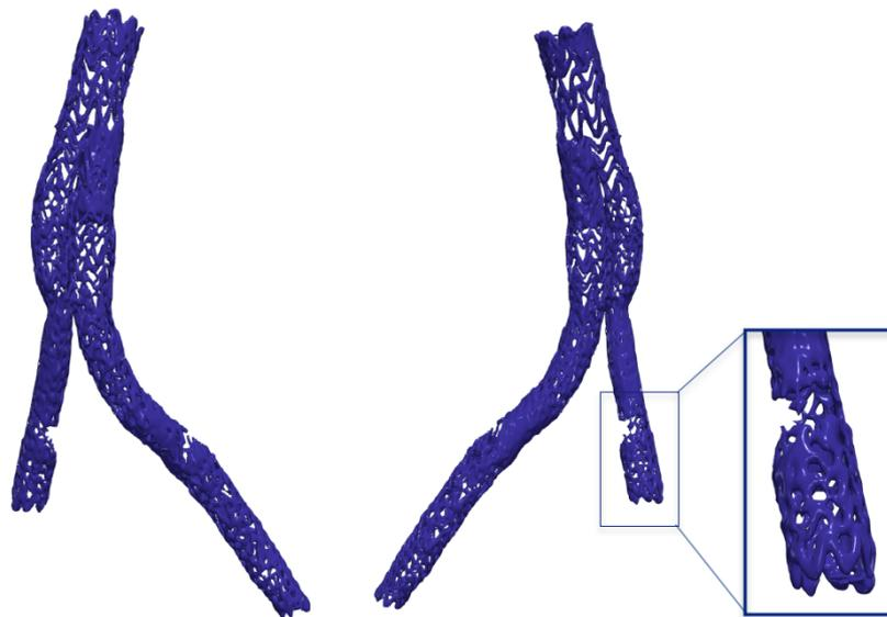
Figure 3.3: PI-T12 segmented stent-graft. A detail of the missing wires of the device is shown in the box.
