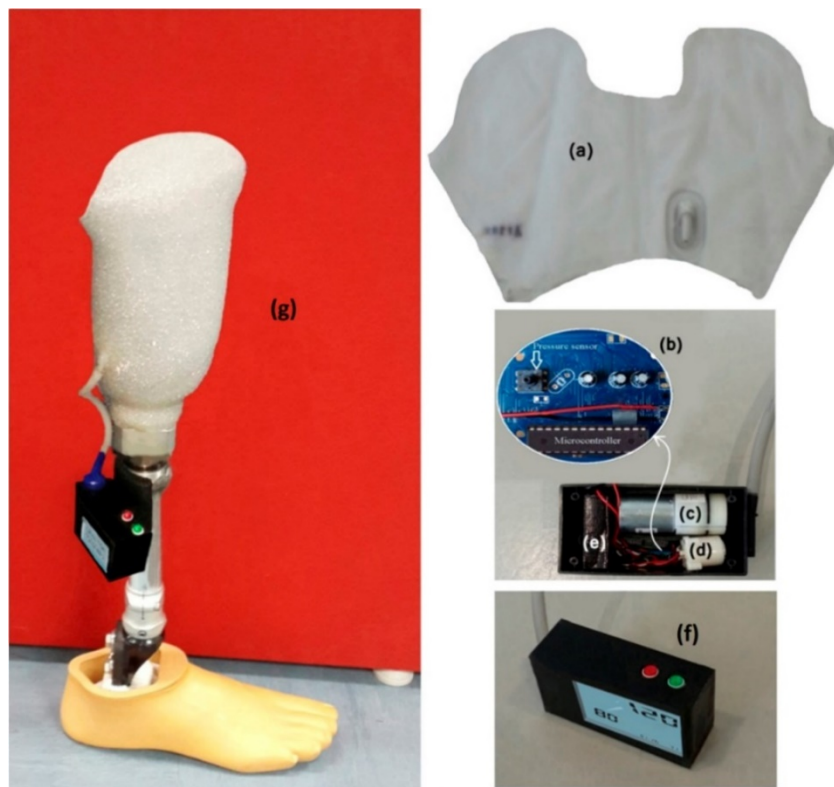
Figure 1-13 The components of APSS: a) Bladder. b) Control circuit board. c) Pump. d) Valve. e) Battery. f) Operation system. g) Assembled transtibial prosthesis
