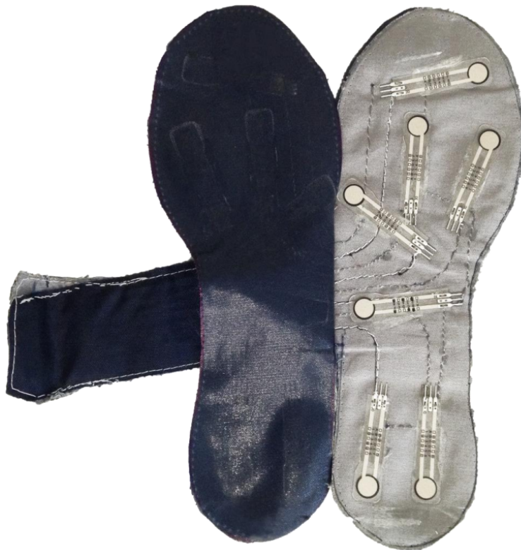
FIGURE 2.1: Opened sensorized insole
