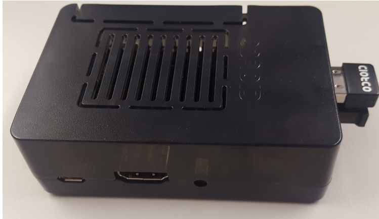
FIGURE 6.2: Odroid microcomputer inside its case.
