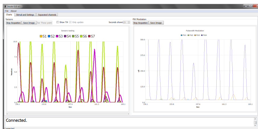
FIGURE 3.1: Real-Time GUI, connected to the server, displaying read values from gait.
