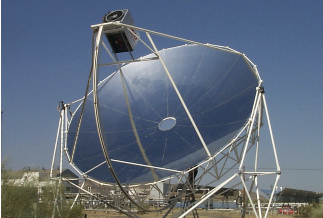
Figure 3: 10kW Solar Dish by Eurodish [5]
