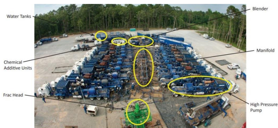
Figure 2-5: Well pad during hydraulic fracturing with trucks carrying pumps for injecting fluids. This evidence the high quantities of required energy. Source: (Drilling Contractor).
