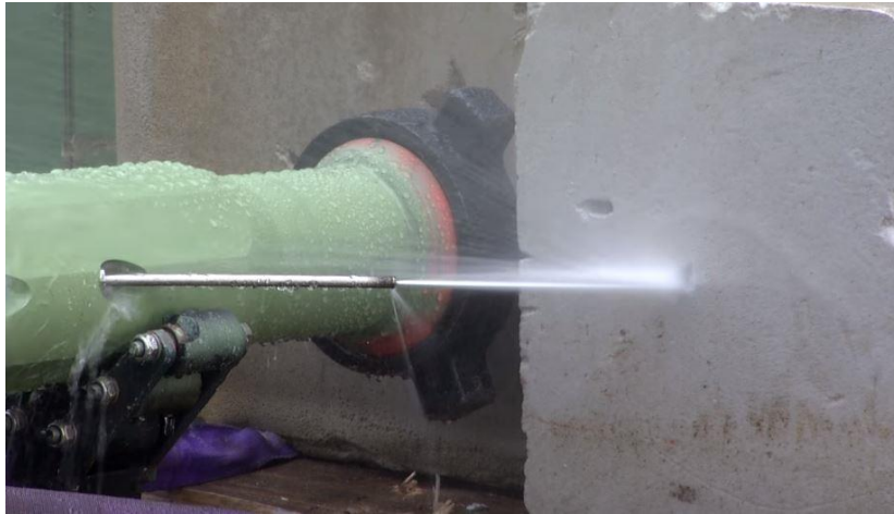
Figure 3-3: Fluid jetting from a lateral during a laboratory test. Source: fishbones.asproducts-2/.
