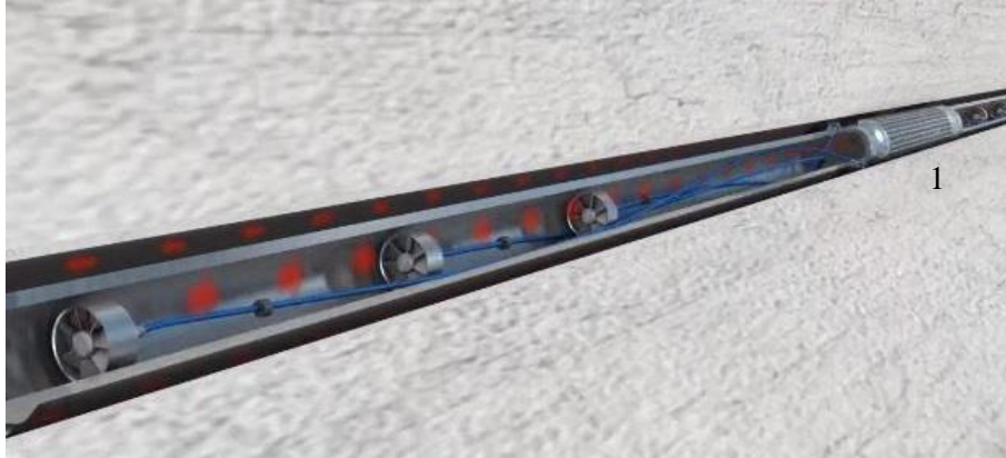
Figure 3-6: Subs alternated with an anchor (1). It is also possible to see the pumped fluid path (red arrows). Source: http://Fishbones.as/videos/ .
