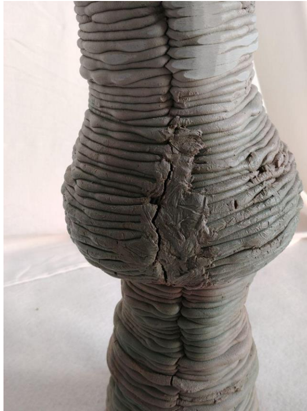
Figure 3.5.4. Close-up on the failure point: as can be observed, the failure started in the discontinuity due to the change of layer
