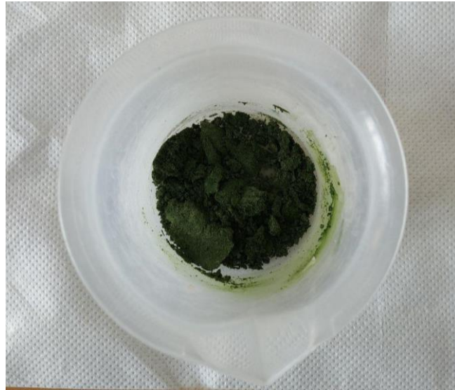
Figure 3.3.53. Mixture obtained with an addition of 7 php of biomass to geopolymer paste containing bentonite. The paste appears discontinuous, even with the addition of supplementary water.
