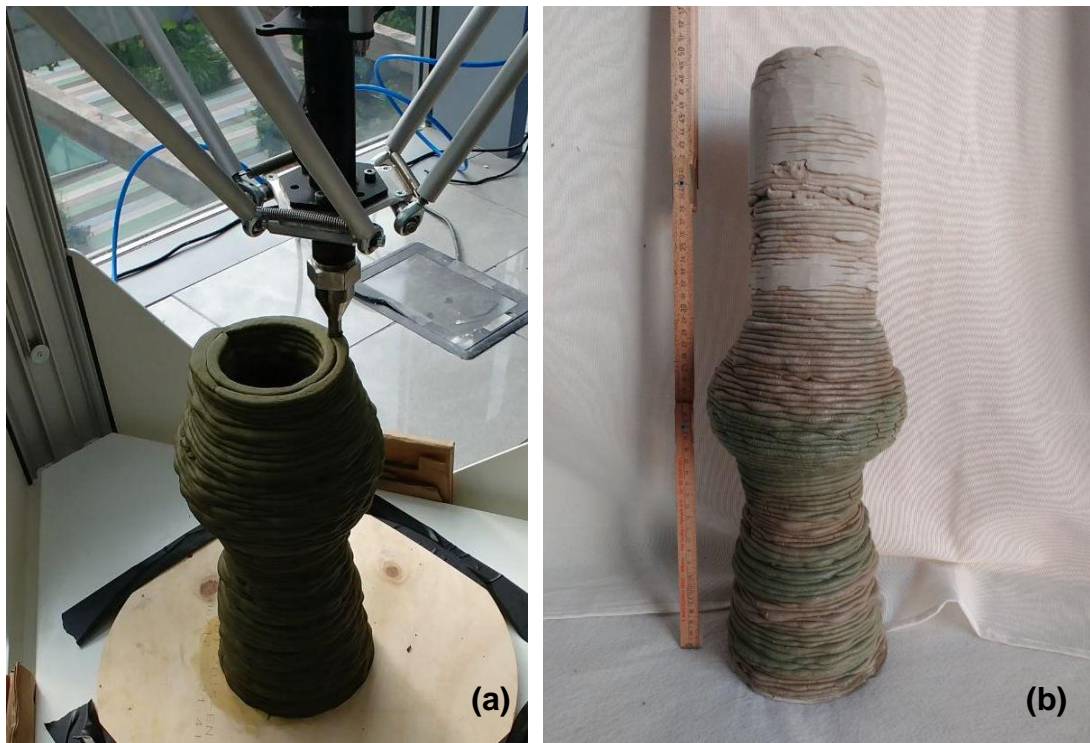
Figure 3.5.3. (a) Printing process of the pipe; (b) final structure, showing a bent shape because of the structural failure occurred
