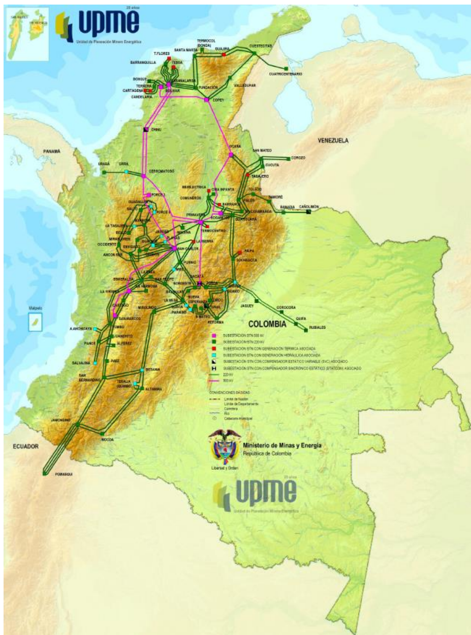
Figure. 51. Colombian National Transmission System in 2016 [17].
