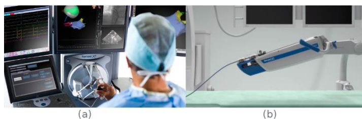
Figure 4. Hansen®'s Sensei Robotic System. (a) Master console. (b) Slave console and the catheter. [10]
