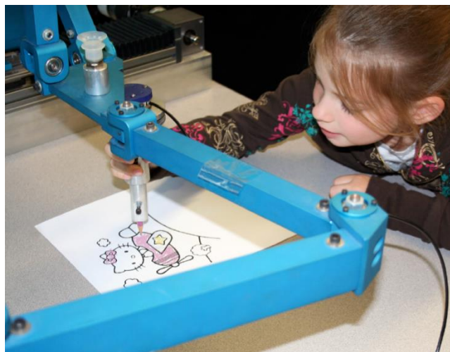
Figure 14. Tripetron 3 DOF planar robot with multi-axes force sensor attached to its end-effector. [17]
