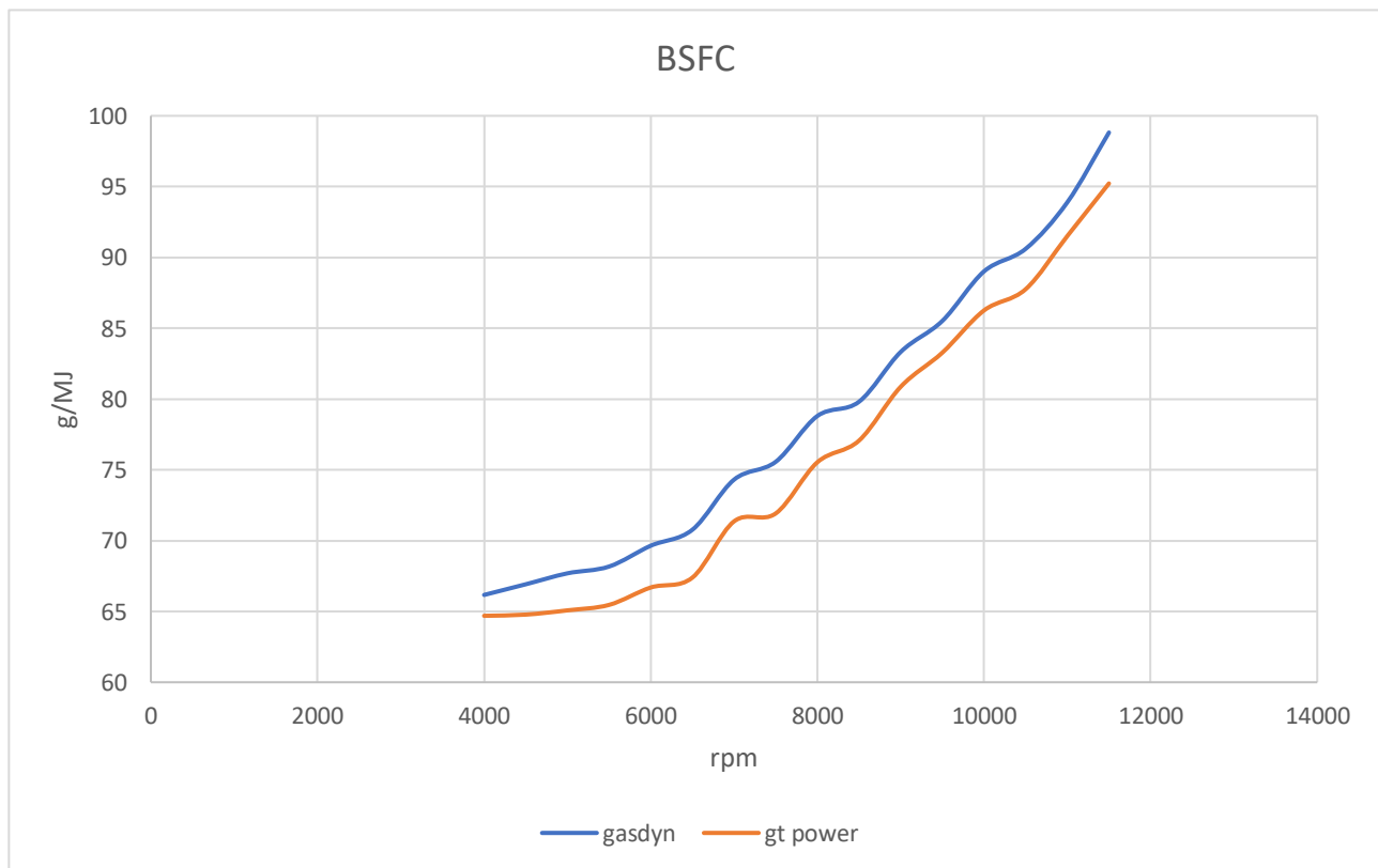
Figure 3.6 Comparison between the specific fuel consumptions provided by Gasdyn and Gt power
