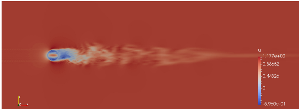
Figure 5.2: u component of the velocity field at 25 time units of simulation. It can be noted that the wake is not fully developed yet. It can also be noted that the velocity is not null inside the sphere.
