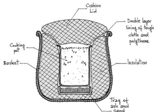
Figure 2.23 Scheme of a haybasket. Source: [2].
