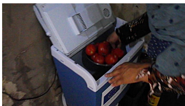
Figure 2.30 Thermoelectric refrigerator powered by the PV system. Credits: the Author.
