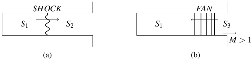
Figure 4.2: unsteady shock propagation through an open-end pipe. Pictures identify the pertinent thermodynamic regions. (a) A shock wave separating zone 1 and 2 is initially moving rightwards; (b) A rarefaction fan separating zone 1 and 3 is traveling leftwards, after the shock is discharged into the infinite-acting reservoir;
