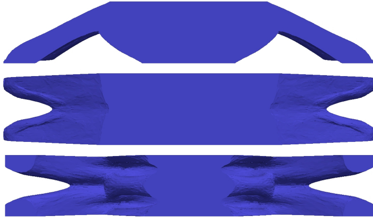
Figure 2.10: The bridge test case (TO): frontal (top), top (center), and bottom (bottom) views of the structure returned by SIMPATY.
