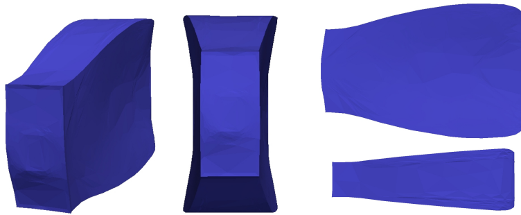
Figure 2.4: The cantilever test case (SO): optimized structure (left), lateral (center), frontal (top-right) and top (bottom-right) views of the optimized structure.
