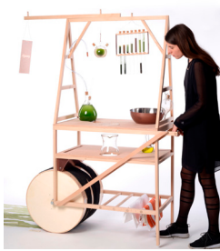
Figure 3.10 Above: DIY aluminum melting machine. Studio Swine.
