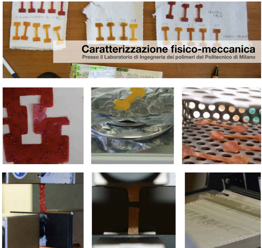
Figure 8.6 DIY-Materials characterized in the Giulio Natta laboratory of Politecnico di Milano.
