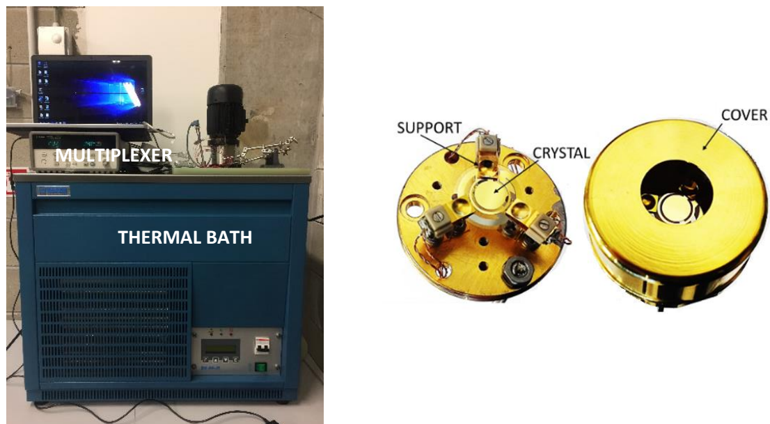
Figure 6 QCM testing setup: (right) detailed view of the crystal mounting structure, (left) overall view of the measurement chain
