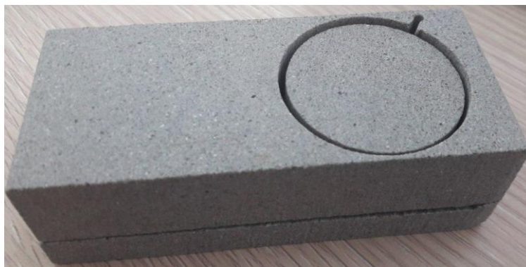
Figure 48. The prepared specimen of Pietra serena sandstone by abrasive water jet technique for dynamic Brazilian disk test.
