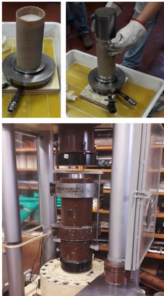
Figure 36. The triaxial testing apparatus (Cividini et al., 1992).
