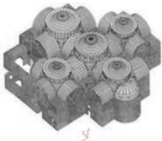
Fig. 2-1 Spatial structural model for FE analysis of Basilica San Marco by Mola et al. (1995)
