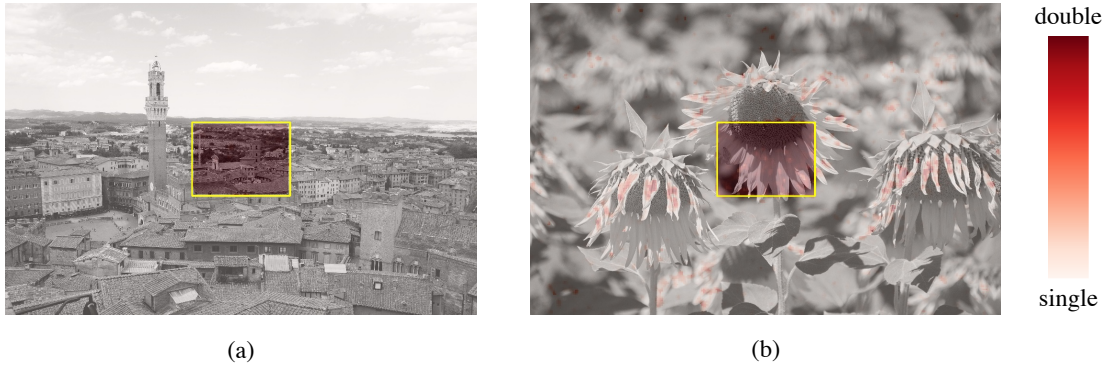
Figure 4.10: A-DJPEG (a) and NA-DJPEG (b) localization example of a compressed central region with QF2 = 95 and QF1 = 80 . \mathcal{C}_{\text{hist}} is used for the aligned case while \mathcal{C}_{\text{noise}} for the non aligned case. Actual forged region lies inside the yellow rectangle.
