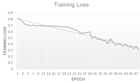
Figure 81. Training loss obtained in a test with 50 epoch, 4 steps per epoch and 1 validation step
