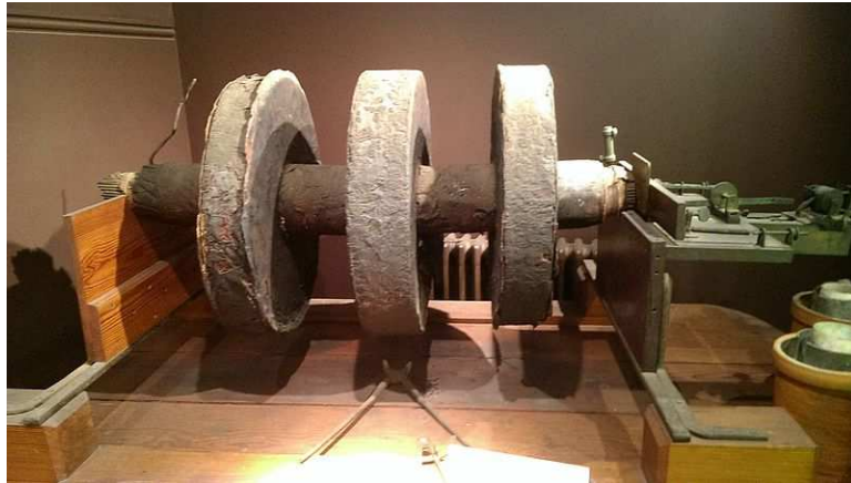
Figure C.10: Clergymen Callan's Induction Coil at the National Science Museum. (Maynooth, Ireland, 1845. Source: Wikimedia Commons).
