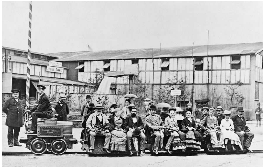
Figure C.15: Exhibition railway with the first electric locomotive (Germany, 1879. Source: Siemens Archives).
