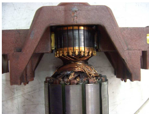
Figure C.5: Commutator and carbon brushes of a DC electrical machine.
