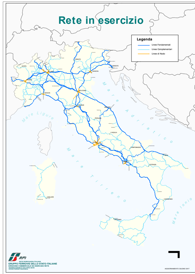
Figure 1.2: Map of railway system in Italy in 2017. More than 70% is electrified at 3kV DC. (Source: rfi.it).
