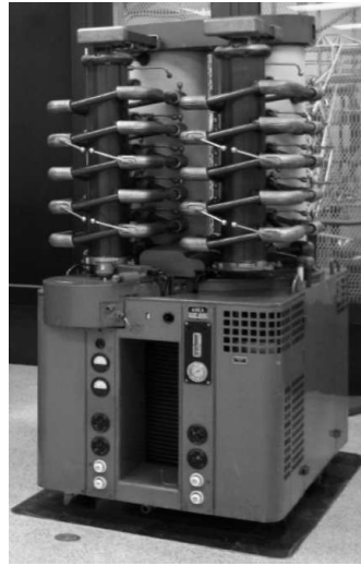
Figure C.24: ASEA-design Mercury-arc rectifier installed in Gotland conversion stations (Sweden, 1954. Source: ABB).
