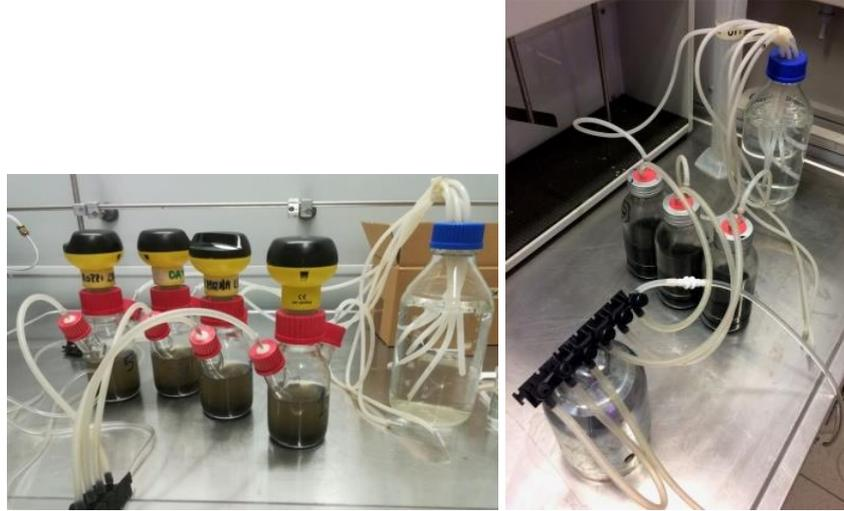
Figure 2. Gas fluxing systems for the OxiTop® (on the left) and for STBs (on the right).
