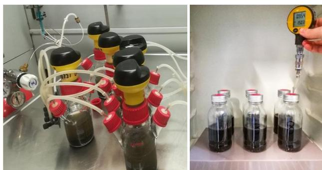
Figure 1. OxiTop® bottle (on the left) and standard bottle (on the right) used in batch tests.
