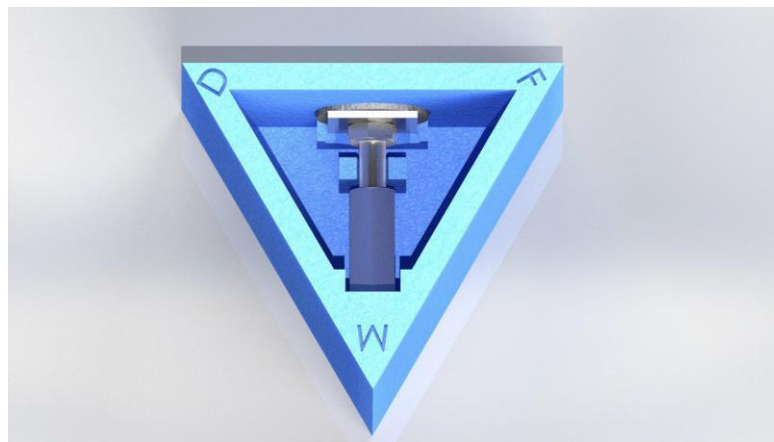
Figure 3.9 Design of the polymeric cell with the sample mounted in.
