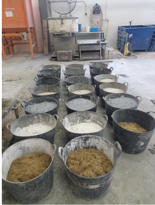
Figure 3-13. Preparation of the materials for UHPFRC mixes
