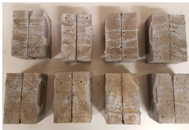
Figure 4–19. Visible chloride penetration in UHPFRC specimens after the spray of silver nitrate
