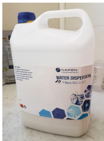
Figure 3–12. Alumina Nano-Fibres from Nafen used as addition in concrete mix
