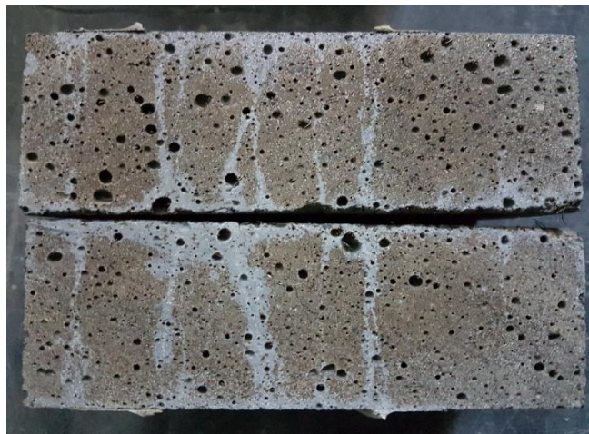
Figure 3–45. Chloride penetration through the specimen thickness (HB4)
