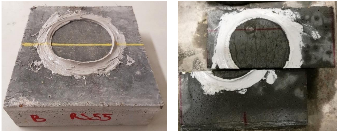
Figure 3–43. Specimen transversely sawn after chloride penetration test
