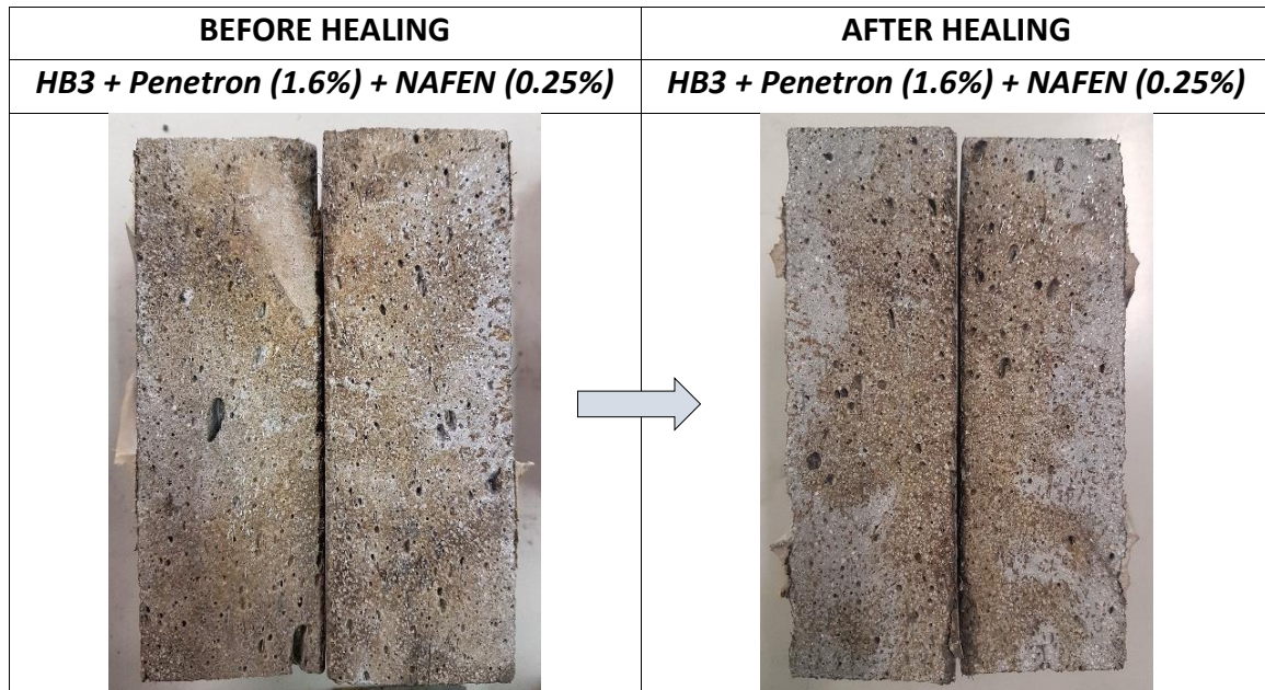
Figure 4–32. Comparison between chloride penetration in HB3 with addition of Penetron (1.6%) and Alumina Nano-Fibres before and after the healing exposure
