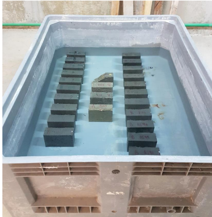
Figure 3-47. Specimens in a tank of water during healing exposure
