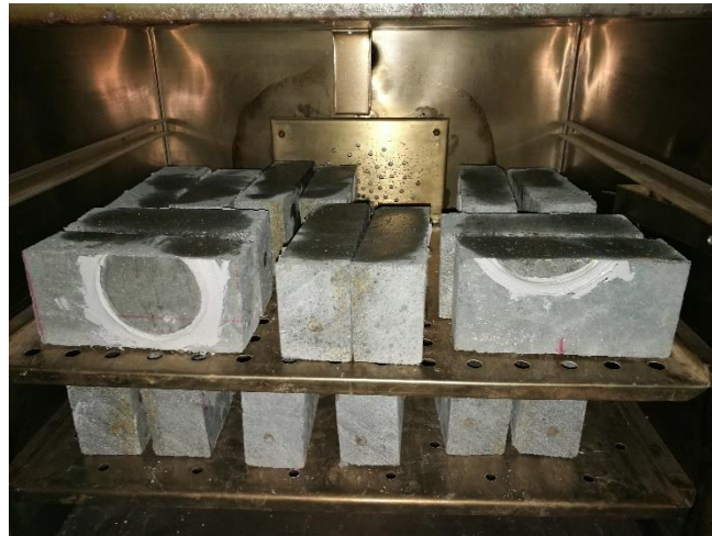
Figure 3–44. Sawn specimens in oven to dry
