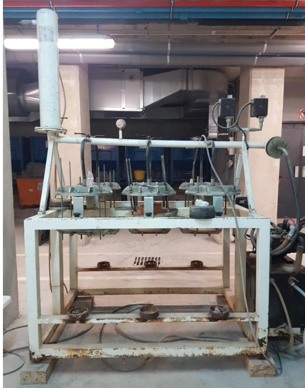
Figure 3–37. Permeabilimeter used for performing high-pressure water permeability tests
