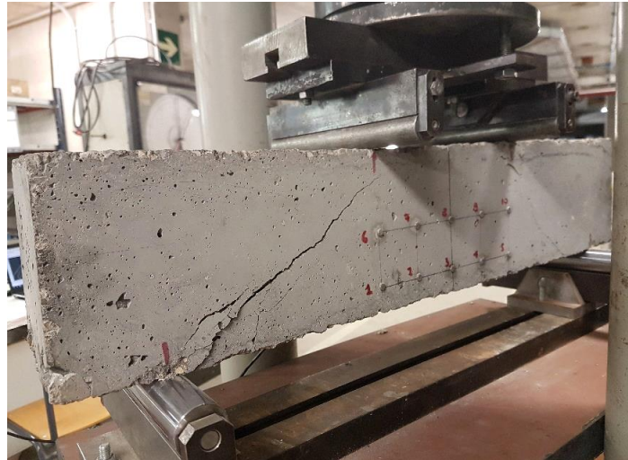
Figure 3–26. Shear crack appeared during pre-cracking
