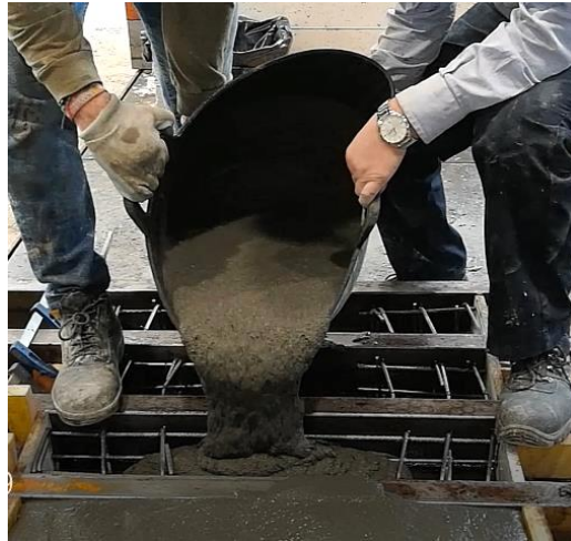
Figure 3-14. Casting into the moulds of base concrete HB3 with self-compacting property
