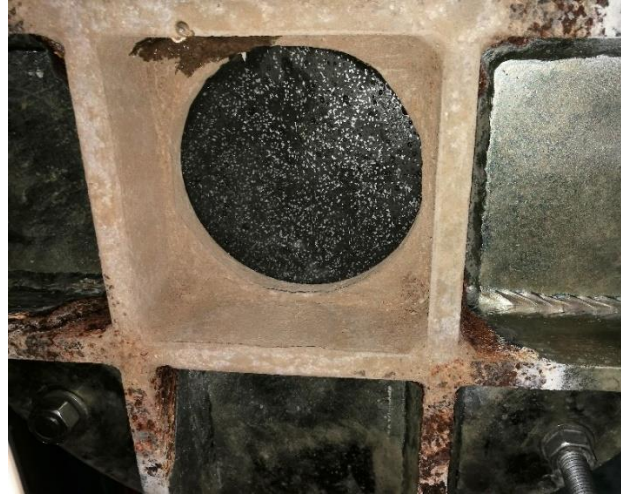
Figure 4-16. Bottom of a UHPFRC specimen during a water permeability test in 2 bar pressure
