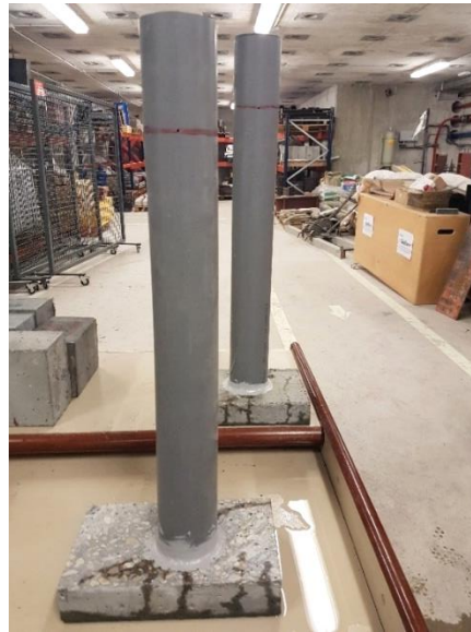
Figure 3–46. Attempt of chloride penetration test with a HPC with 0.3 mm of crack width
