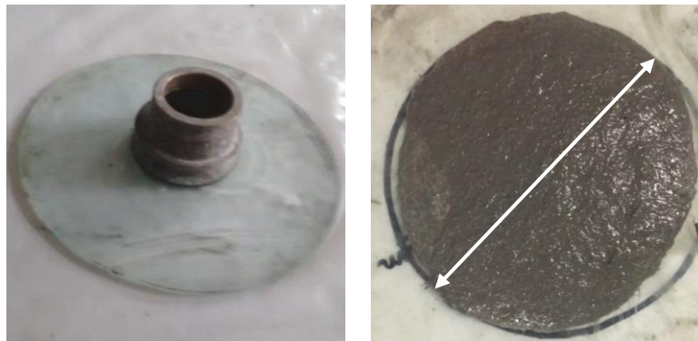
Figure 3-15. Mini-cone workability test in UHPFRC base mixes
