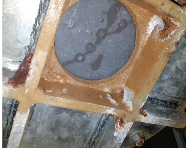
Figure 3–39. Drops of water from a 0.05 mm crack during high-pressure water permeability test
