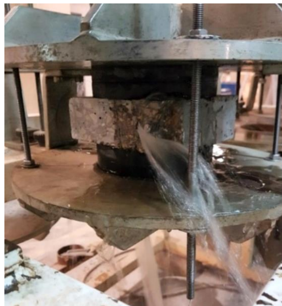
Figure 3–40. Leakage of water from a side crack during the high-pressure water permeability test in a traditional concrete
