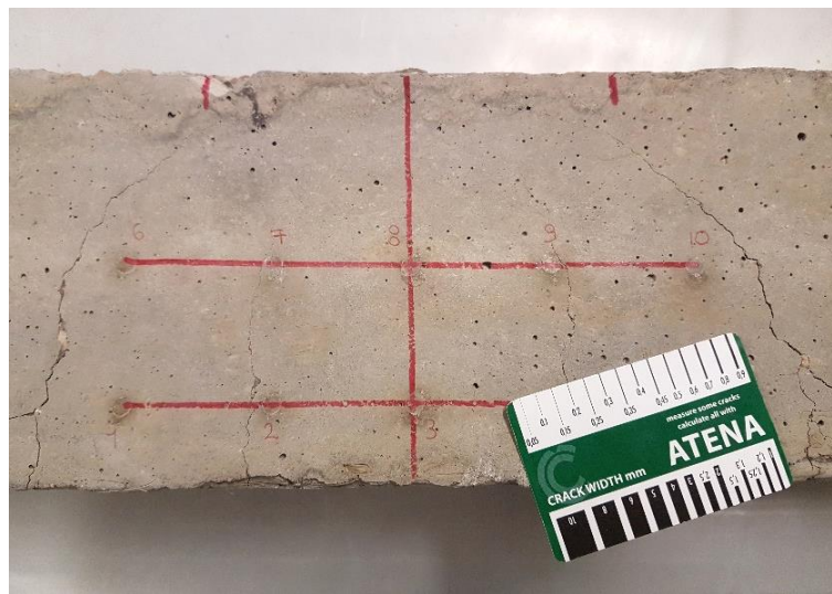
Figure 4–11. Traditional concrete cracking pattern with few localized cracks
