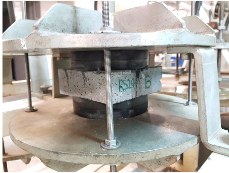
Figure 3–38. High-pressure water permeability test methodology
