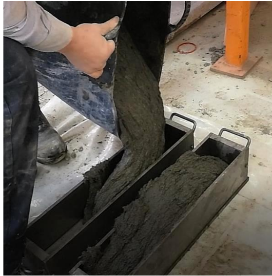
Figure 3–16. Lack of workability when using HB3 + 2.4% of Penetron Admix
