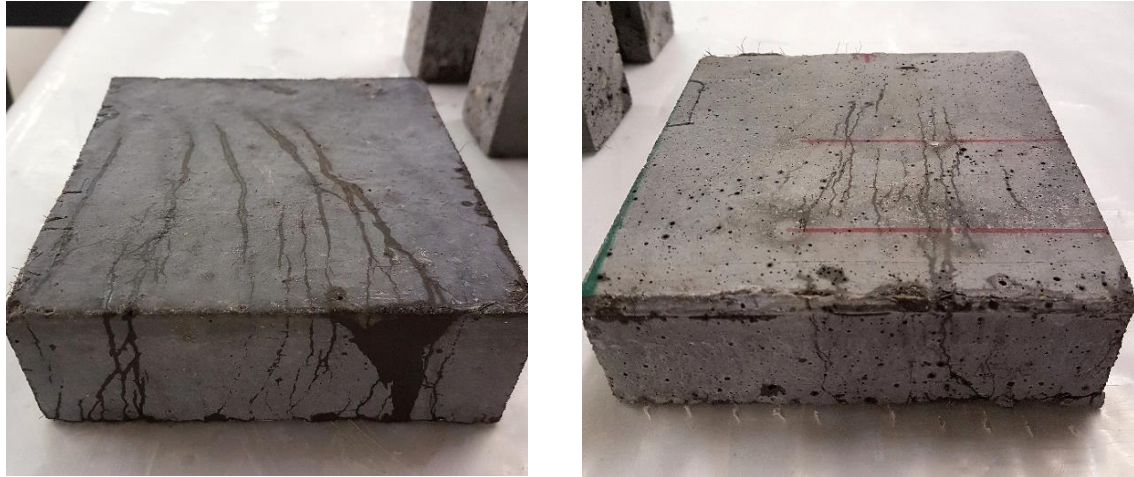
Figure 4–17. Cracks made visible by the water permeability test
