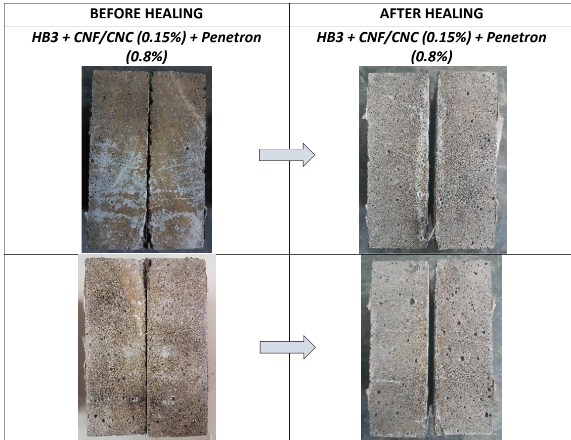
Figure 0-7. Self-healing outcome HB3 + CNF/CNC (0.15%) + Penetron (0.8%)
