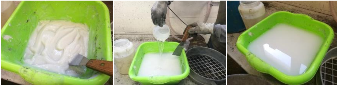
Figure 3–11. Dilution of Nanocellulose in tap water
