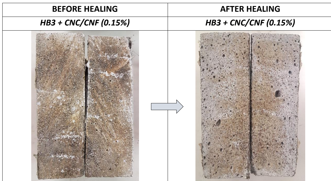
Figure 4–31. Comparison between chloride penetration in HB3 with addition of Nanocellulose before and after the healing exposure
