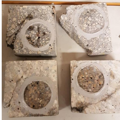
Figure 4–18. Specimens after low-pressure water permeability test
