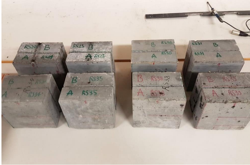
Figure 3-36. Specimens A and B obtained after sawing
