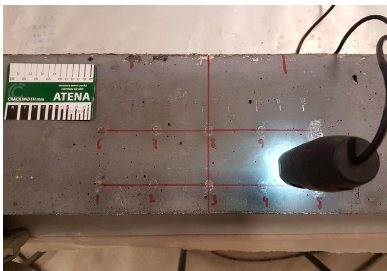
Figure 4–12. UHPFRC cracking pattern with multiple micro-cracks
