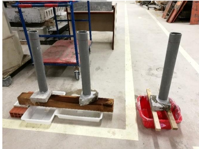
Figure 3-41. Low-pressure water permeability test methodology
