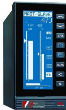
Figure 3.3: PLC multi-loop controller.
