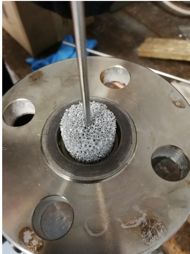
Fig. 4.9: Foam loading into the reactor.
