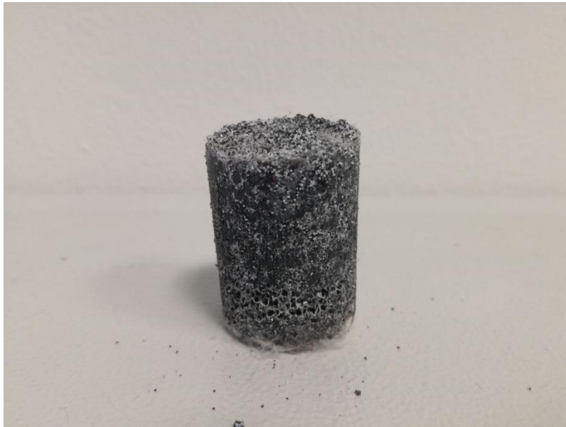
Fig. 4.21: Foam and spent catalyst removed from the reactor.
