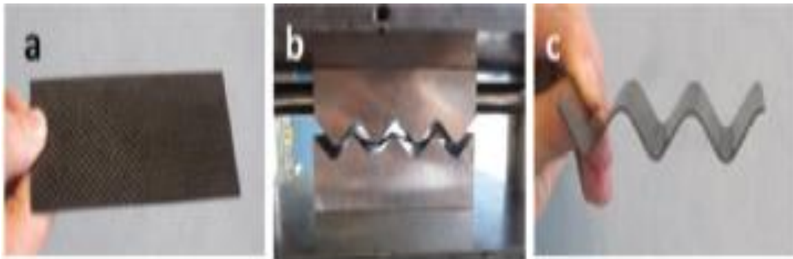
Figure 1.3.18. Thermoforming of a cured composite laminate [50]
