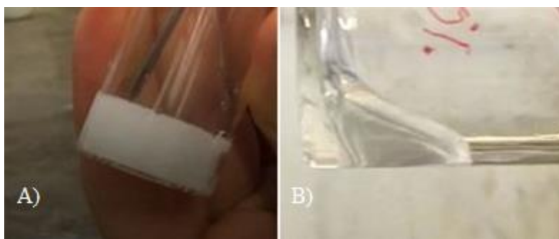
Figure 49: Samples with A) and without B) EGDMA, after 1 h at 60°C.
