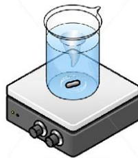
Figure 44: Rotation field created by a magnetic stirrer
