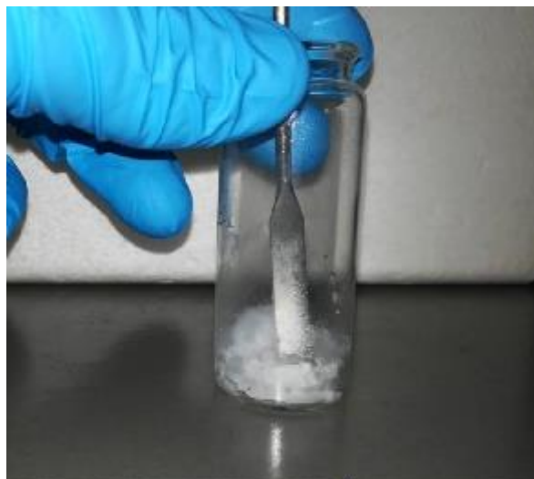
Figure 50: Fragmentation of the solid polymer using the initiator AAPH.
