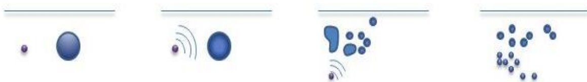
Figure 46: Sonicator ultrasound waves that break the monomer droplet.
