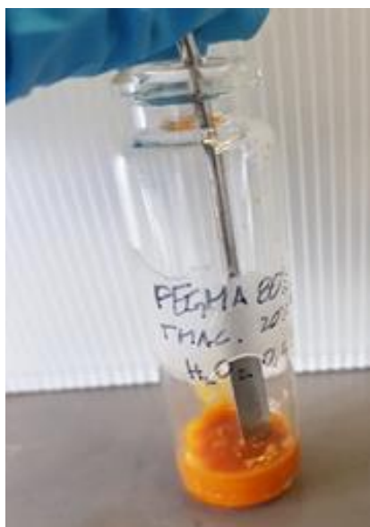
Figure 52: Result using TMAEMC and PEGMA 500 and H 2 O 2 at 10%.
