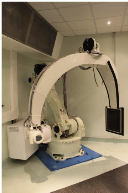
Figure 13. Custom robotic in-room imaging (CBCT) installed in the central room of CNAO. Source: Rossi, 2015
