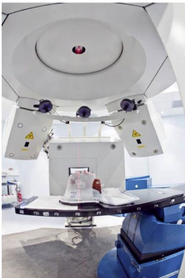
Figure 12. Patient positioning and verification system inside one of treatment rooms at CNAO. Source: Rossi, 2015
