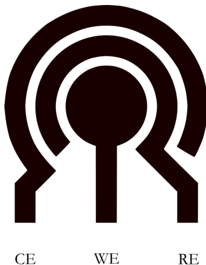
Figure 2.1: Design of the three-electrode setup for amperometry.
