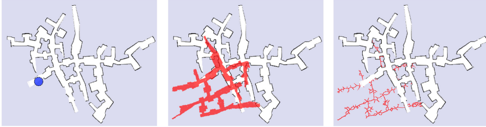
Figure 2.9: The figure illustrates the loop-closure prediction. Left: map explored so far with the frontier under consideration (blue dot). Middle: One of the predictive belief (red) superimposed on the map. Right: Voronoi diagram. From [30].
