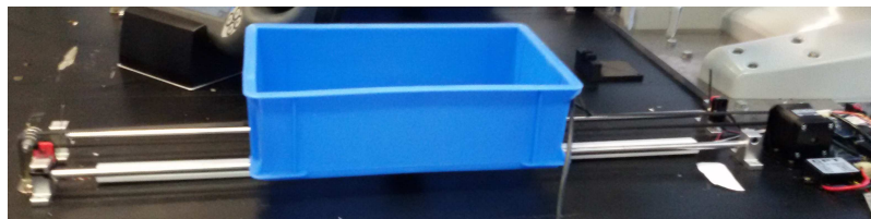
Figure 2.1: Photo of the Mechanical System. The blue box is connected to the linear guides through the bearings. It is connected to the motor by belt and pulley transmission. The stroke is limited by the limit switches.
