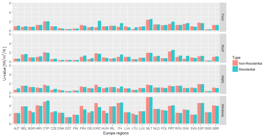
Figure 2.3: Country-level U-values of different envelope components, for the residential and non-residential sector (European Commission database)
